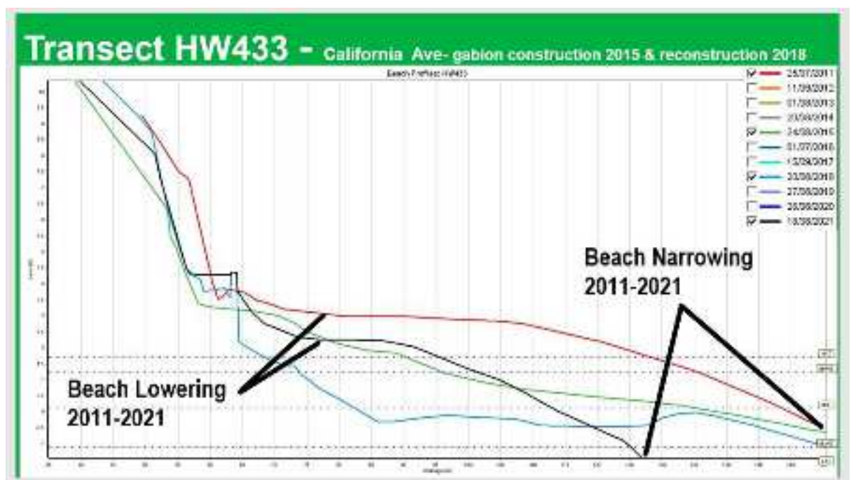
Figure 6 Anglian Coastal Monitoring Programme Beach Level Data, 2011, 2015, 2018 and 2021, for transect HW433 in the immediate vicinity of the Scratby damaged gabions
