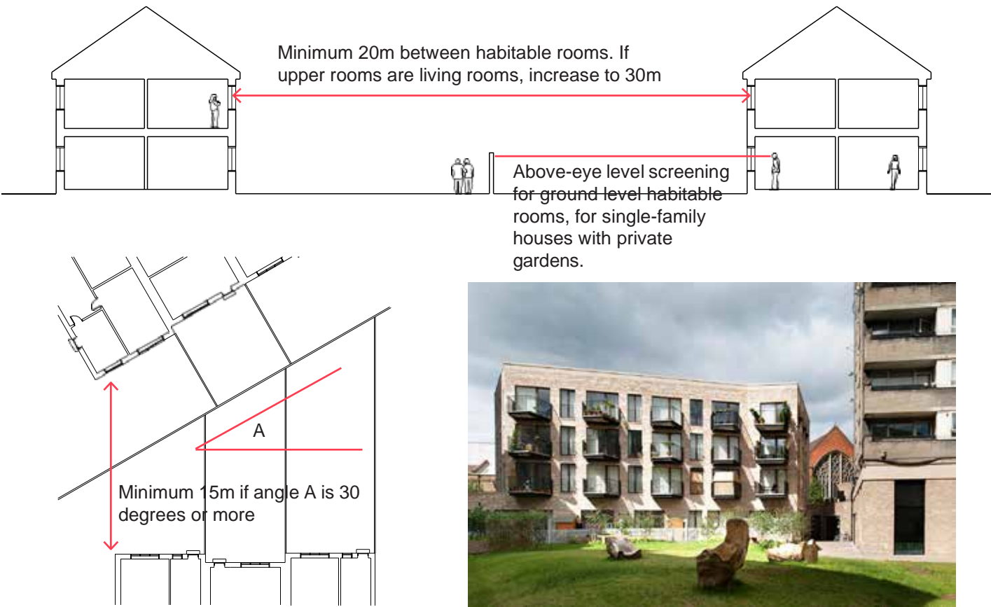
Fig. 40. Diagrams showing parameters for privacy at the rear of new homes and example of apartment building where above-eye-level rear screening is not require, and distances can be reduced, for rear windows and balconies overlooking shared private amenity space, at the Silchester Estate (Architect: Haworth Tompkins)
