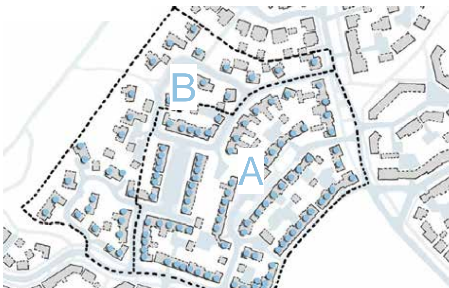
Fig. 36. Diagram from the National Model Design Code showing how to measure site density. Note that the area boundaries go to the centre-line of streets and to the rear of plots, and do not include significant areas of public open space. Area A has a higher density than area B.
