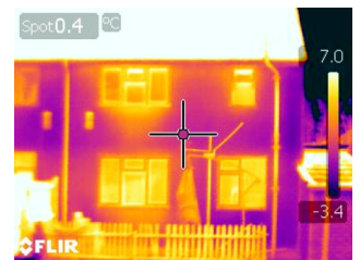
Thermal image of the building prior to work commencement, bright colours indicate high heat losses from central heating radiators
