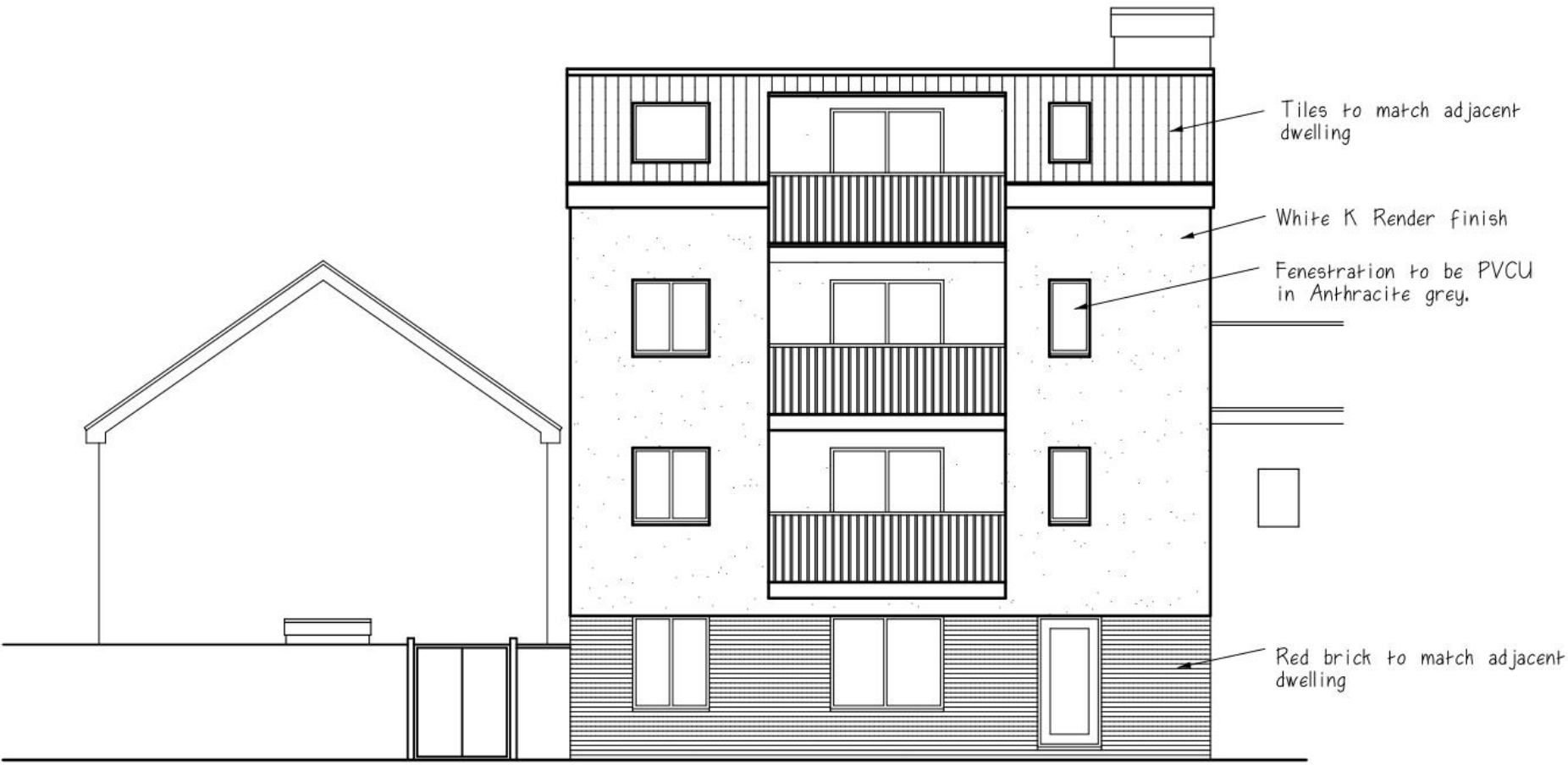
PROPOSED WEST ELEVATION 1:100
