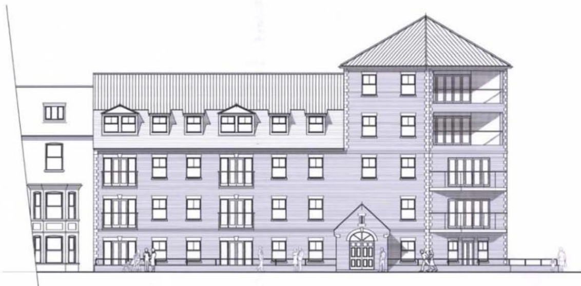
PROPOSED EAST ELEVATION 1:100
