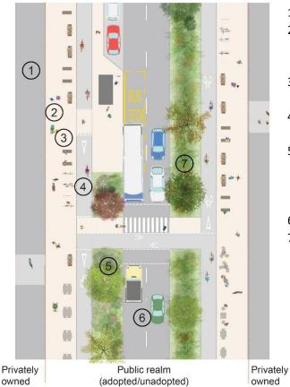
Examples of High Street with cycle tracks, SuDS, trees and seating alongside necessary vehicle traffic.
