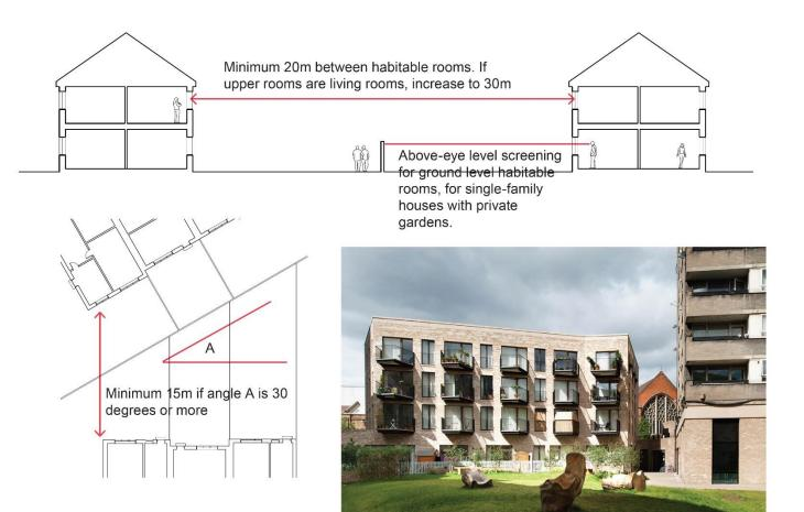
Figure 44. Diagrams showing parameters for privacy at the rear of new homes and an example of an apartment building where above-eye-level rear screening is not required, and distances can be reduced, for rear windows and balconies overlooking shared private amenity space, at the Silchester Estate (Architect: Haworth Tompkins).
