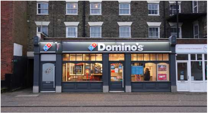
Fig. 053 An example of integrated lighting, which is sympathetic to the fascia and doesn't dominate visually.
